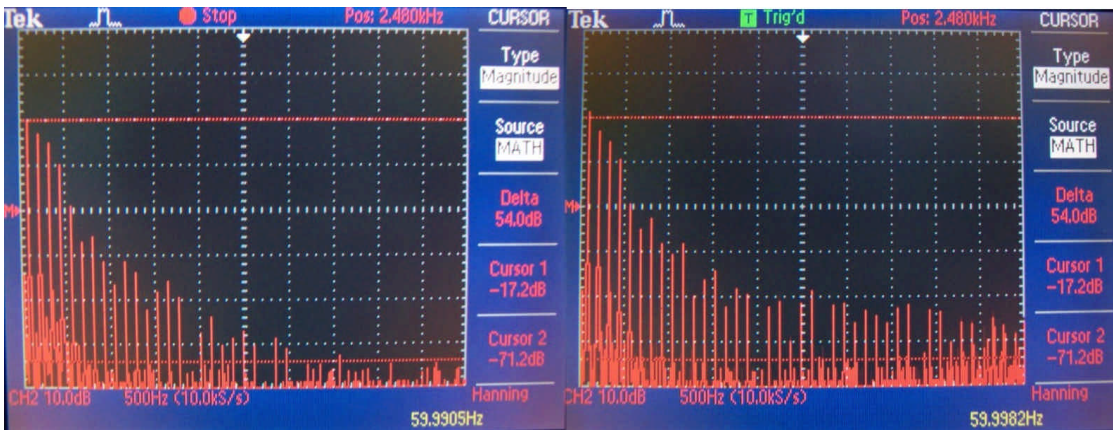
Figure 12, Spectra of load current before (left side) and after (right side) Stetzer filter was plugged-in. Frequency spans are from 0 Hz to 5 kHz.
